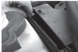
16. Reinstall the base on the left hand side of the cowling and then slide the screw into the base.
